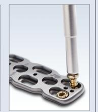
Remove drill guide and use a self-tapping bone screw to tighten into plate
